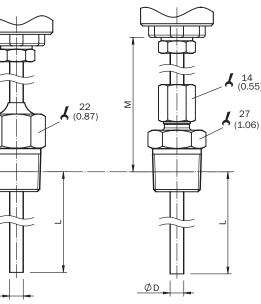
Dimensional drawing: housing, without process connection
