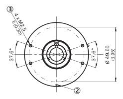
XF7 values see shaft diameter table for blind hollow shaft
