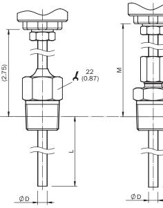
Dimensional drawing: housing, without process connection
