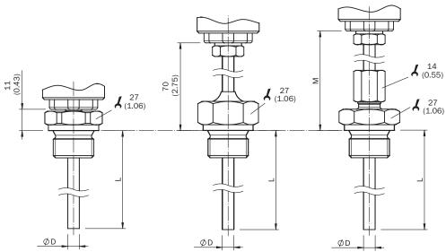
Dimensional drawing: conical threads
