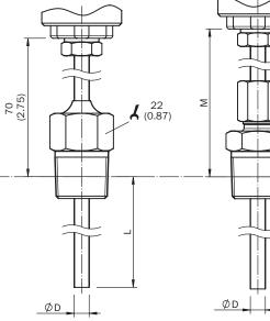
Dimensional drawing: housing, without process connection
