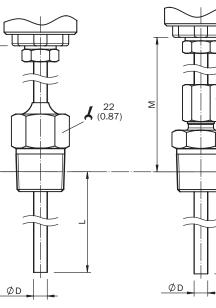
Dimensional drawing: housing, without process connection
