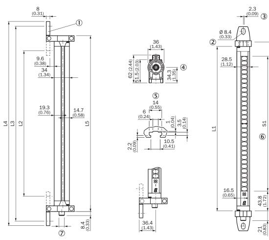
Sender with swivel mount, small housing (receiver mirror image)
