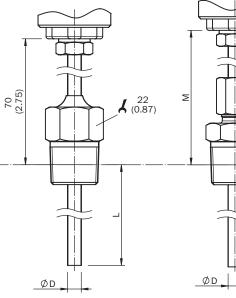
Dimensional drawing: housing, without process connection
