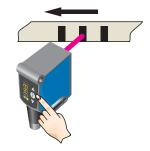
Press the Set pushbutton to end the teach-in process.
