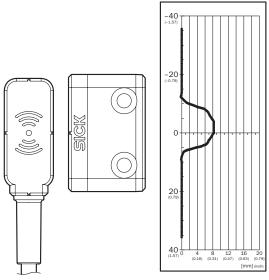
Safe switch on distance  $S_{\text{ao}}\,6\,\text{mm}$
