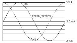
Signal diagram for clockwise rotation of the shaft looking in direction "A" (see dimensional drawing)1 period =  $360^{\circ}$ :  $1024^{\circ}$  Signal diagram for clockwise rotation of the shaft looking in direction "A" (see dimensional drawing)1 period =  $360^{\circ}$ :  $1024^{\circ}$
