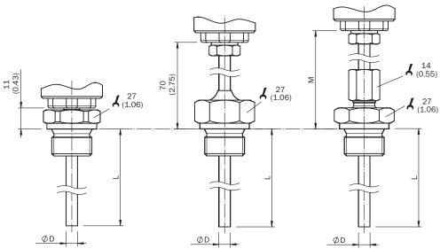
Dimensional drawing: conical threads
