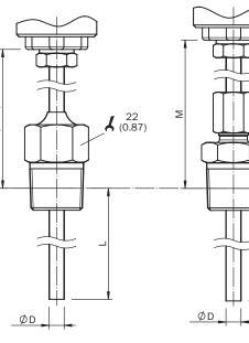
Dimensional drawing: housing, without process connection
