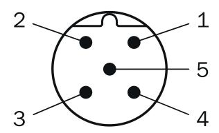
Male connector M12, 5-pin, A-coded
