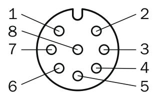
Female connector M12, 8-pin, A-coded
