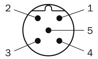
Male connector M12, 5-pin, A-coded
