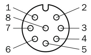
Female connector M12, 8-pin, A-coded
