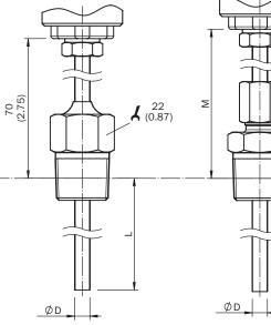
Dimensional drawing: housing, without process connection
