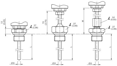
Dimensional drawing: conical threads
