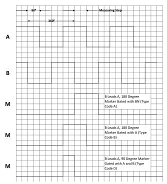
Cw with view on the encoder shaft in direction "A", compare dimensional drawing. Signal Outputs with Clock-wise Counting Direction Option Selected (A leads B for clock-wise rotation). Complement signals AN, BN and ZN are not shown.
