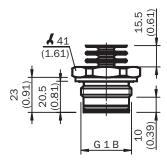
Housing with L-connector (DIN EN 175301-803 A)
