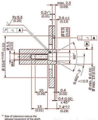
\*) Size of tolerance reduce the allowed movement of the shaft, see data sheet.
