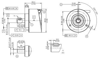
① Operating temperature measuring point (freely selectable, around the housing surface area in each case, approx. 3 mm away from flange)
