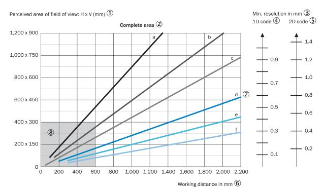
Min. resolution in mm  $\Im$ Perceived area of field of view: H x V (mm) 1D code ④ 2D code (5) Narrow area (8) 400 x 300 а 0.35 b - 0.3 - 0.4 300 x 225 С - 0.25 - 0.3 - 0.2 200 x 150 d  $\overline{7}$ 0.15 - 0.2 е - 0.1 100 x 75 f - 0.1 - 0.05 0 0 100 200 300 400 500 600 Working distance in mm 6a: f = 8.0 mm (C-mount standard only) 9d: f = 25.0 mm e: f = 35.0 mm b: f = 12.0 mm - c: f = 16.0 mm f: f = 50.0 mm
