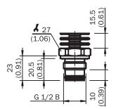
Housing with L-connector (DIN EN 175301-803 A)
