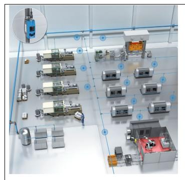
The SICK FTMg flow sensor can be positioned to identify leaks based on pressure losses, thereby minimising the operating costs for producing, supplying and distributing compressed air.
